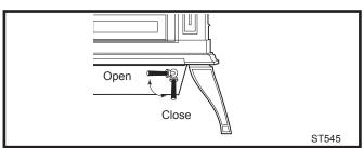
Fig. 27 Turn the handle to the ash pan compartment clockwise to open and counterclockwise to close.
